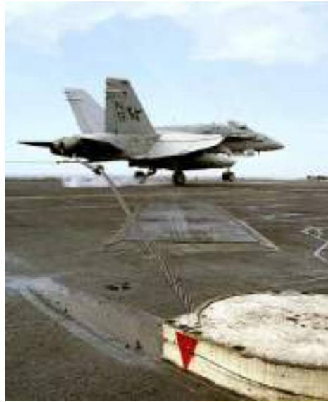
Figure 1.C-4: Tailhook and arresting wire on an aircraft carrier.
