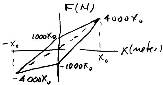
Given suspension force vs  $x$  indep of  $\omega$ ,  $M = 10\text{kg}$ .
