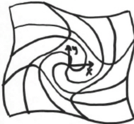
Figure 1.34: Deformation of a grid by an irrotational vortex, \psi = C \ln(\sqrt{x^2 + y^2}) .
