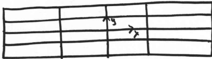
Figure 1.32: Deformation of a grid by a stagnation flow, \psi = Axy . In general, grid spacing will be closer near origin and larger far from origin; this is not terribly clear from the sketch.
